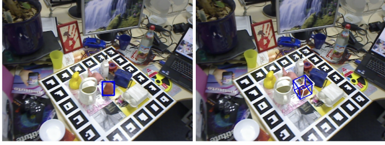
Figure 12: Result of the 6D pose estimation done by G2L_net
